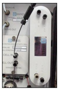
Figure B-20. Suppressor Installed (SRS Shown)
