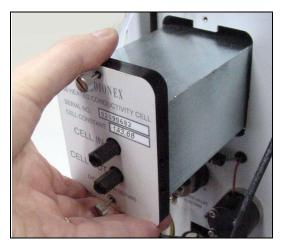
Figure 5-15. Removing the Cell Assembly
