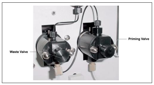
Figure 5-12. Waste and Priming Valves
