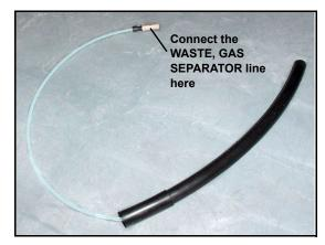
Figure B-21. Gas Separator Waste Tube Assembly
