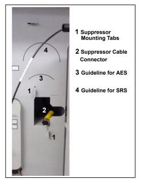
Figure B-19. Suppressor Mounting Tabs and Guidelines
