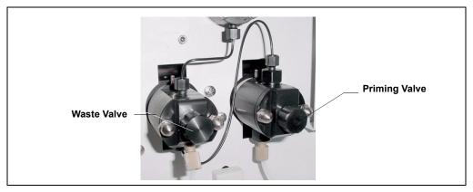
Figure 4-2. Waste and Priming Valves
